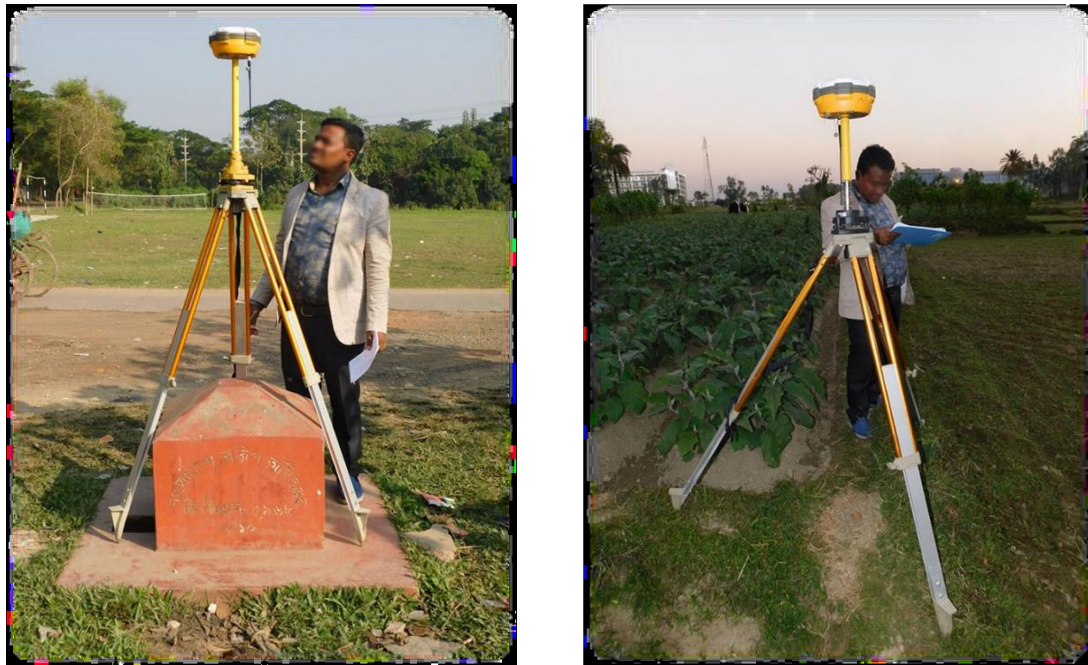
Figure 5-4: RTK Base Station, SOB Geodetic Pillar (Left) and RTK Survey at Corner of a Plot (Right)
